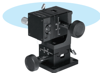
TLM-412+TSS-401+TTS-413 TLM-412 units with a travel amount of \pm 10 mm and a TTS-413 goniometer stage have been combined. A compact X/Z tilt stage structured on a 40 mm x 40 mm stage.
